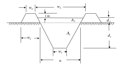
Design a water canal that has a wet-section cross sectional area (area of the cross section occupied by water,  $A_1+A_2$ ) of at least 150.0  $m^2$ . For safe passage of boats, the water depth in the canal,  $d_1 + d_2$ , must be larger then 15 *m*. Least construction cost occurs when the volume of the excavated material,  $A_1$ , equals the amount of material used for the dykes as shown in the figure above.
